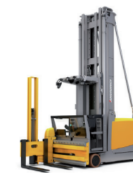
F1 | Rider | Electric Very narrow aisle lateral (& front) stacking trucks - operator up
