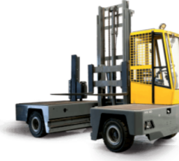
C1 | Rider | Electric & I.C.E. Side loader up to & including 5 tonne
