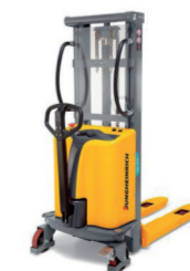
Z3 | Pedestrian | Manual & Semi Manual Pallet stacker
