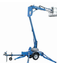
1B | Rider & Pedestrian | Electric & I.C.E. Static boom - trailer mount, van mount, lorry mount & spider lift, cannot drive elevated
