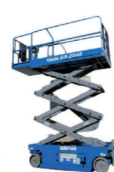
3A | Rider | Electric & I.C.E. Mobile vertical - can drive elevated
