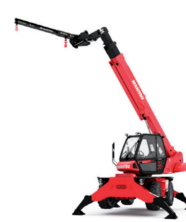
J6 | Rider | I.C.E. Variable reach/tele, 360° slew under 9m lift
