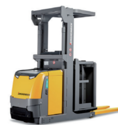
E1 | Rider | Electric Medium lift order picking trucks up to 2.5m
