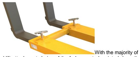
forklift attachments being of the fork-mounted variety (where the operator drives the forks of the forklift into the pockets of the attachment) it's important to ensure the sizing of the attachment fits that of the forklift truck. For example, using fork pockets that are too large for the forks, any securing methods on the attachments could be compromised.
