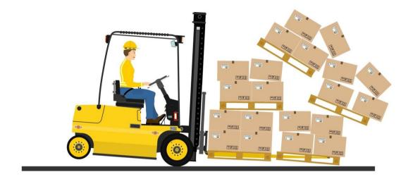
When fitting a forklift attachment, the capacity of the forklift truck is affected. This is known as the 'De-Rated' capacity. The weight of the attachment, combined with the weight of the product to be handled and the distance from the attachment to the forklift truck will all have a bearing on the forklift's lifting capacity. It's important, therefore, that you check how your attachment will affect your truck's safe handling capacity. If in doubt, always check with your forklift supplier.
