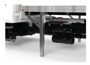
The support leg is only securely locked when the leg brace and the spring bolt pin are engaged.
