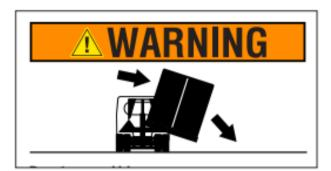
19. An improperly secured container that falls off a chassis can result in injury or death. It is the driver's responsibility to make sure that the container is properly locked onto the chassis before each trip.
