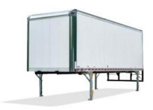
Demountable containers, standard truck bodies equipped with retractable legs.
