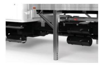
The support leg is only securely locked when the leg brace and the spring bolt pin are engaged.
