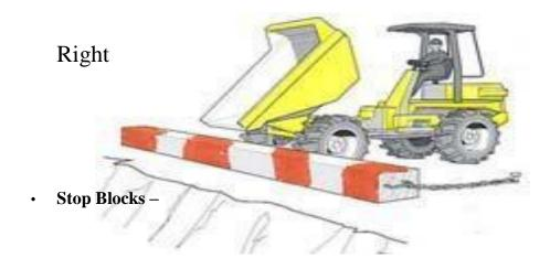
• provide a physical barrier to help prevent the dumper rolling into the trench when tipping.
