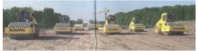
Combination Rollers Sheep's Foot and Smooth Drum
