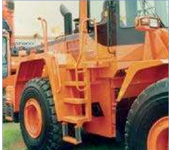
Figure 18 Access to vehicles – steps and handrails
