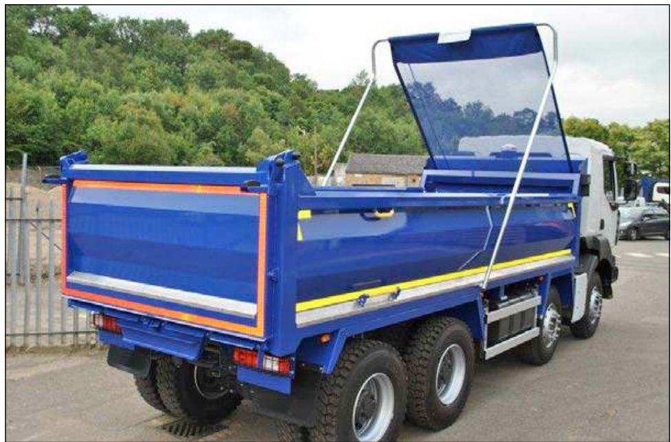
Figure 20 Front-to-rear sheeting system
