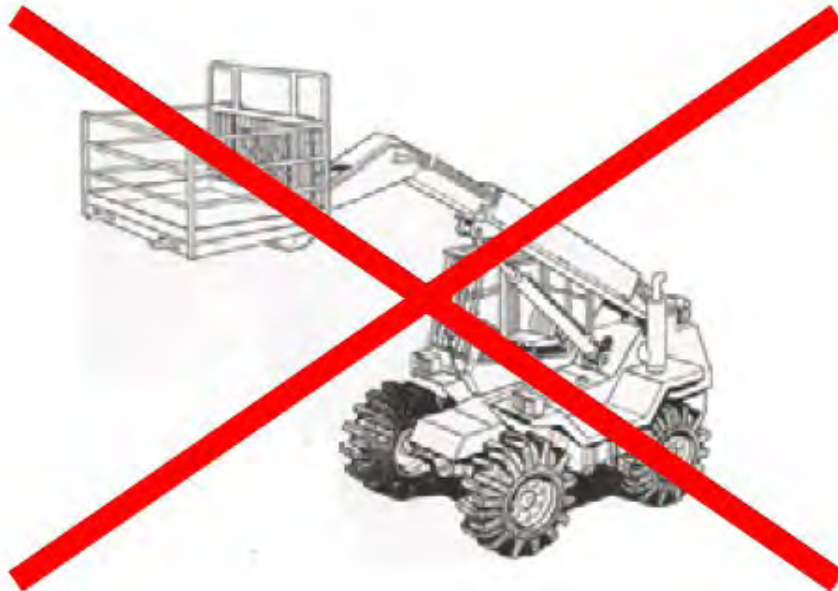
Figure 27 - Non-integrated Work Platform
