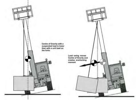
• Figure 9 - Lateral Stability for Suspended Loads
