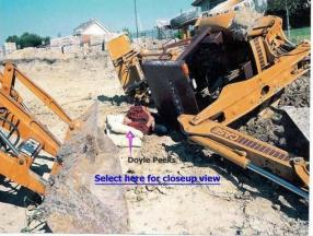
• Sideways Rollovers Can Happen- When the Excavator is driven across steep slope, driving too close to excavations or edges, working or lifting cross track, overloading, lifting full loading buckets at full reach
