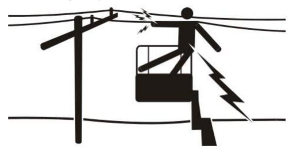
This machine is not insulated and does not provide protection from contact or proximity to electrical current.
