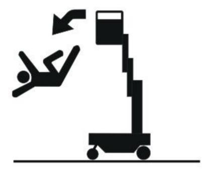
Keep both feet firmly positioned on the platform floor at all times. Never use ladders, boxes, steps, planks, or similar items on platform to provide additional reach.
