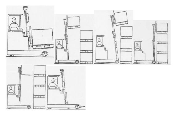
When the fork arms are clear of the stack, re-apply the parking brake, engage neutral if the reach truck has been moved. Lower the forks into the travel setting and check the way is clear before moving off.
