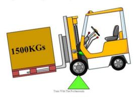
DO NOT leave a gap between the heel of the forks and the front side of the load, this will increase the load centre, and could cause the truck to tip forward.
