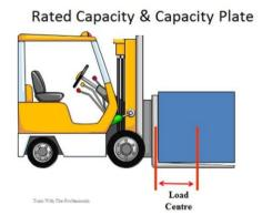
The lift trucks "rated capacity" applies with the mast in the vertical position, this also applies with the manufactures stated lifting capacity.
