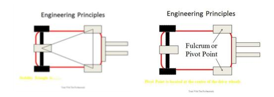
The stability triangle is between the front drive wheels and rear wheel on a three wheel truck or middle of the rear axle on a 4 wheel truck
