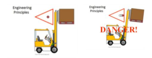
DO NOT tilt the mast forward at height! Tilting the load forward at height will move the "Combined centre of gravity forward, and could cause the truck to tip"
