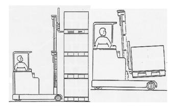
It is important that the forks are horizontal when they are run in under the pallet. They must not be forced in,but must run freely. Carrying the pallet, after an incorrect in section results in the entire weight of load being borne by a single board, which might then break.
