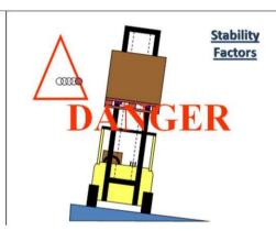
While this may look safe, it is a dangerous manoeuvre; as soon as you raise the load it also raises the combined centre of gravity of the truck and the load and moves it out of the stability triangle
