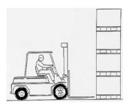
Look upwards to check for clearance, raise the fork arms to a position permitting clear entry into the pallet. The forks should be nearer to the top of the entry point in order to compensate for the taper of the forks.
