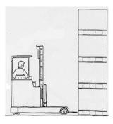
Halt approximately 6" to 12" from the stack and apply the parking brake and engage neutral. Bring the mast to the vertical position or ensure the forks are level. If necessary adjust the fork arm spread to suit the width of the load and ensure that the weight of the load is within the capacity of the reach truck.
