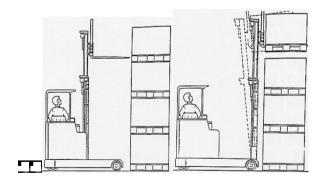
Lower the load carefully and smoothly to the correct travelling position. Apply sufficient back tilt to stabilise the load before checking the way is clear and moving off.
