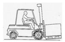
Approach the stack, square, in the correct travel position with the load low.
