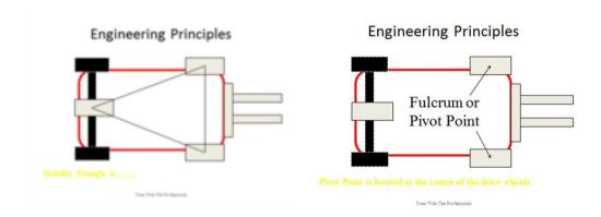
The stability triangle is between the front drive wheels and rear wheel on a three wheel truck or middle of the rear axle on a 4 wheel truck
