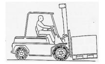
Approach the stack, square, in the correct travel position with the load low.
