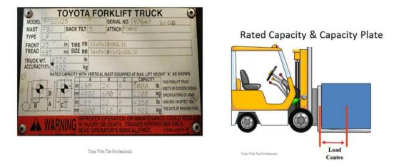
The lift trucks "rated capacity" applies with the mast in the vertical position, this also applies with the manufactures stated lifting capacity.
