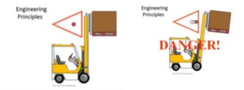
DO NOT tilt the mast forward at height! Tilting the load forward at height will move the "Combined centre of gravity forward, and could cause the truck to tip"
