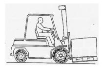
Approach the stack, square, in the correct travel position with the load low.
