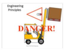
DO NOT tilt the mast forward at height! Tilting the load forward at height will move the "Combined centre of gravity forward, and could cause the truck to tip"
