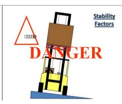
While this may look safe, it is a dangerous manoeuvre; as soon as you raise the load it also raises the combined centre of gravity of the truck and the load and moves it out of the stability triangle
