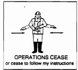
The signaller should stand in a safe place where he can see the load and can be seen clearly by the driver. Face the driver if possible. Each signal should be distinct and clear.
