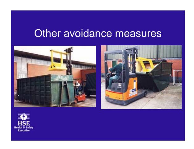
Takes out the need to access height to flatten down loads or deal with overhanging loads
